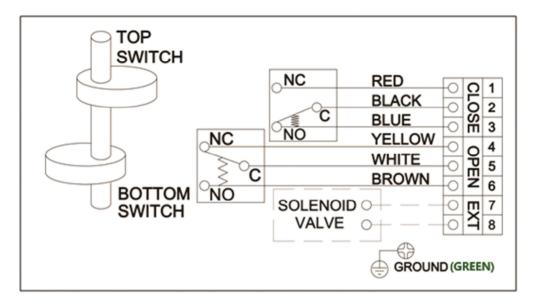
MECHANICAL SWITCH (3 SPDT)
