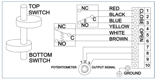
Mechanical Switch (2 SPDT) with Signal Unit
