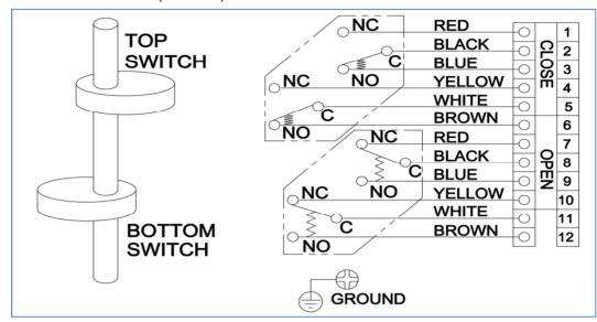
⑤ Mechanical Switch (2 SPDT) with Potentiometer
